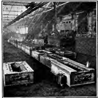
Fig. 64. Completing Moulds Ready for Pouring.
